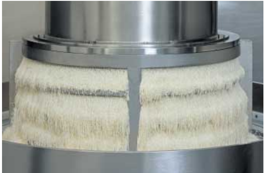
Production of stable and uniform extrudates
