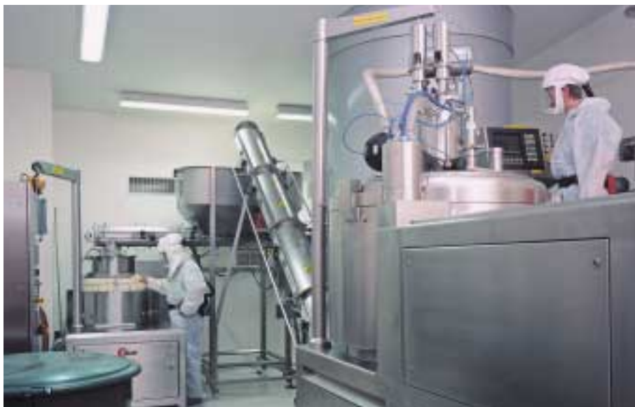
Extrusion line consisting of a vertical granulator and a basket extruder
